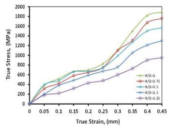
Figure 6: True Stress-Strain for Solid Lubricated Specimens
