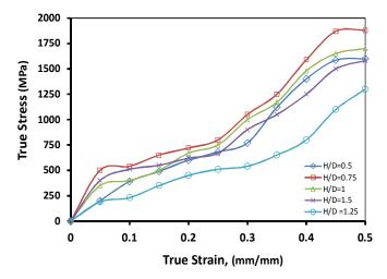
Figure 5: True Stress-Strain for Solid Non-Lubricated Condition
