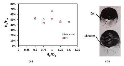
Figure 3: (A) Deformation Ratio of Tapered Specimens at Various aspect Ratios H<sub>0</sub>/D<sub>0</sub> (B) Tapered Specimens after Compression Test
