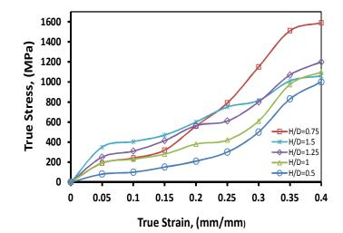
Figure 7: True Stress-Strain for Tapered Non- Lubricated Specimens
