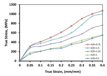
Figure 9: True Stress-Strain for Collar Non-Lubricated Specimens
