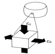
Figure 1: Localized Strains on the Bulging Cylindrical Surface of a Compression Test Specimen
