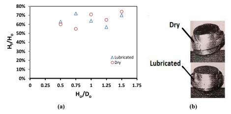
Figure 4: (a) Deformation Ratio of Collar Specimens at Various aspect Ratios H<sub>0</sub>/D<sub>0</sub> (b) Collar Specimens after Compression Test
