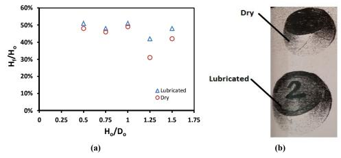
Figure 2: (A) Deformation Ratio of Solid Specimens at Various Aspect Ratios  $H_0/D_0(B)$  Solid Specimens after Compression Test
