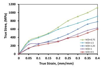
Figure 10: True Stress-Strain for Collar Lubricated Specimens
